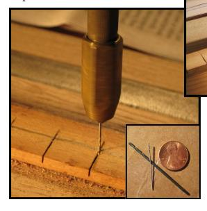
A .025" hole is next drilled in the hammer butt spring rail for the tail of each spring to be inserted through. (The insert shows the size of this drill bit in comparison to a penny, and an ordinary 1/16" bit.)
