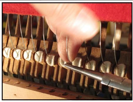
A new set of original-type springs being given final adjustments in the action.
