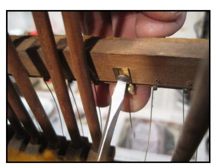
Although supply catalogues claim this is an easy repair ("Quickly installed in any upright action without removing the spring rail. . ."), it can be a very aggravating job when the small part has to be installed amidst all the other parts. (In the photo, adjacent hammer assemblies and the hammer rest rail have been removed for clarity.)
