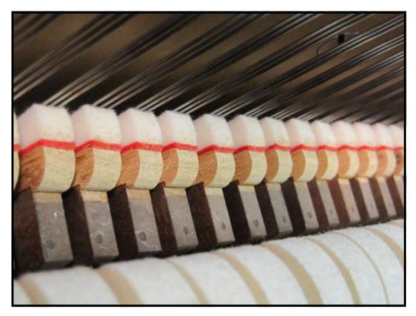
A new set of treble dampers installed and ready quiet things down when needed.
