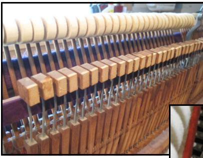
Once all the dampers have been removed, and the dampers blocks have been reinstalled, it is time to return the action to the piano.
