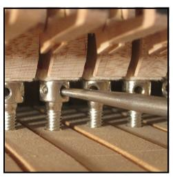
Adjustment of capstans to raise or lower hammer height. Hammer height refers to the distance from the striking surface of the hammers to the underside of the strings. This is set at the optimum distance for the hammer to swing to achieve maximum power. Just as the amount of swing is important to a golfer when he hits the ball, too little or too much swing when a note is played on the piano is not desirable.
