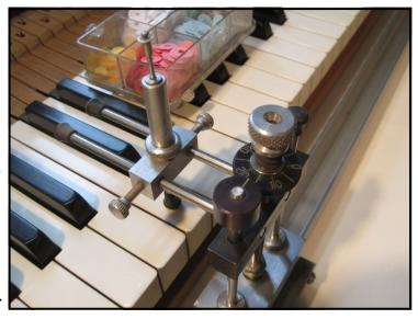
refining the mechanism by going through the complete series of steps a number of times until everything is at the optimum setting.
