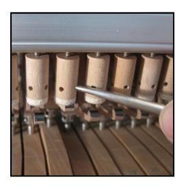
Adjustment of letoff buttons. The letoff button releases the mechanism in its upward motion a split-second before the hammer reaches the strings. This way, the hammer is traveling under its own momentum when it hits the strings, and is not just shoved into them. This adjustment is made such that the hammers release as close to the strings as possible so that when the pianist plays with an exceedingly light touch, the piano will respond.
