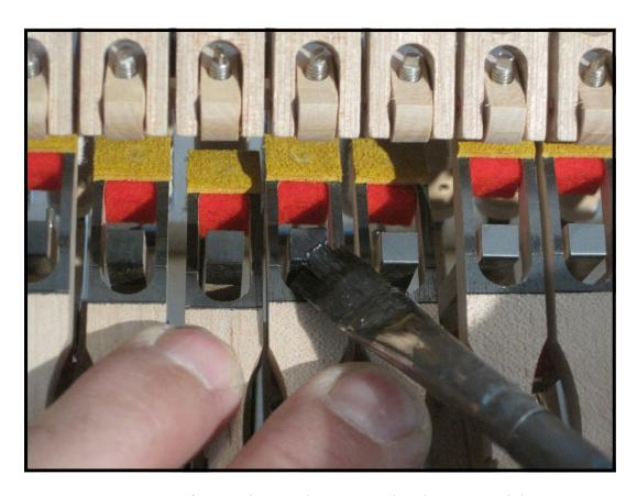
Friction points of a grand action being coated with an action lubricant.
