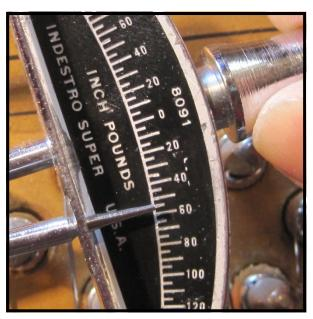
The above photos show torque reading measurements done on the same tuning pin before and after treatment was administered. In the photo on the left, the untreated pin measures just under 20 inch pounds of torque. After a single treatment the pin measures a much better reading of 55 inch pounds of torque.
