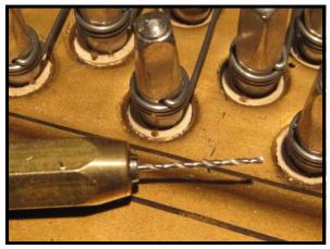
Sometimes if the tuning pin bushing is very tight, it may be necessary to drill a tiny hole through each bushing to allow the liquid to seep down to the pinblock. The drill in the photo to the left measures a mere .025", small enough to drill a hole in the thin wooden bushing surrounding each tuning pin. By drilling this hole, the liquid can better penetrate to where it's needed.
