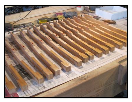
The new tops are glued to the keysticks with a special adhesive which produces a rock solid bond between the keytop material and the wooden keystick. This type of glue creates a bond stronger than the wood itself.
