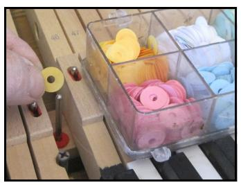
Once the measurement has been made for the key, leveling papers are added at the balance rail to bring the height of the key up to level. Papers as thin as .001" are used to produce a perfectly level set of keys. After all the keys have been leveled, the leveling papers and the balance rail felts will be flipped so that the felts are on top.
