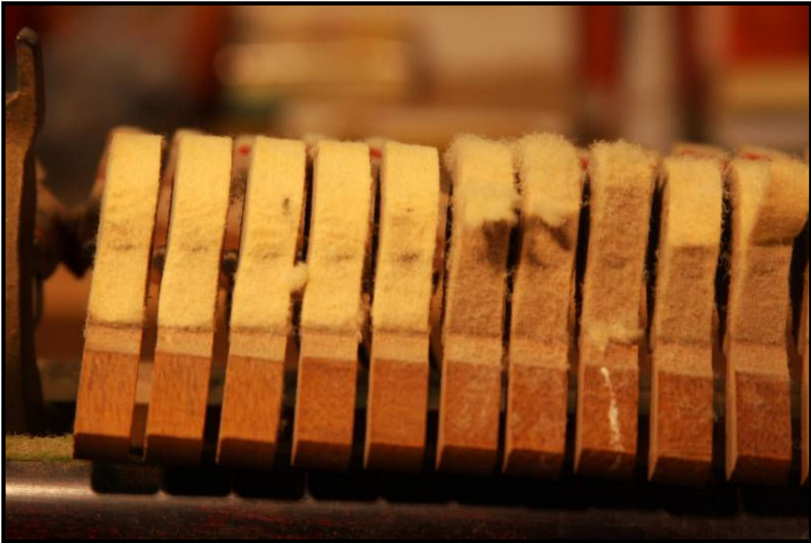
Hammers in the process of being filed - good felt underneath coming to light
